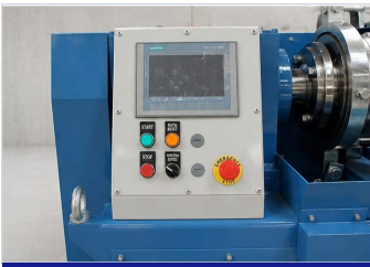
SIEMENS PLC / HMI KONTROL
